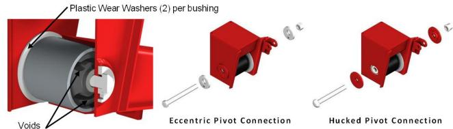
Bushings can normally be inspected from underneath the trailer without disassembly. The following is the recommended initial check.
